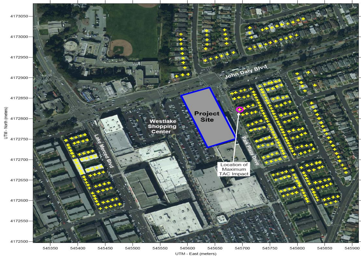
Figure 4.3-1: Project Construction Site and Locations of Off-Site Sensitive Receptors and Maximum TAC Impacts
