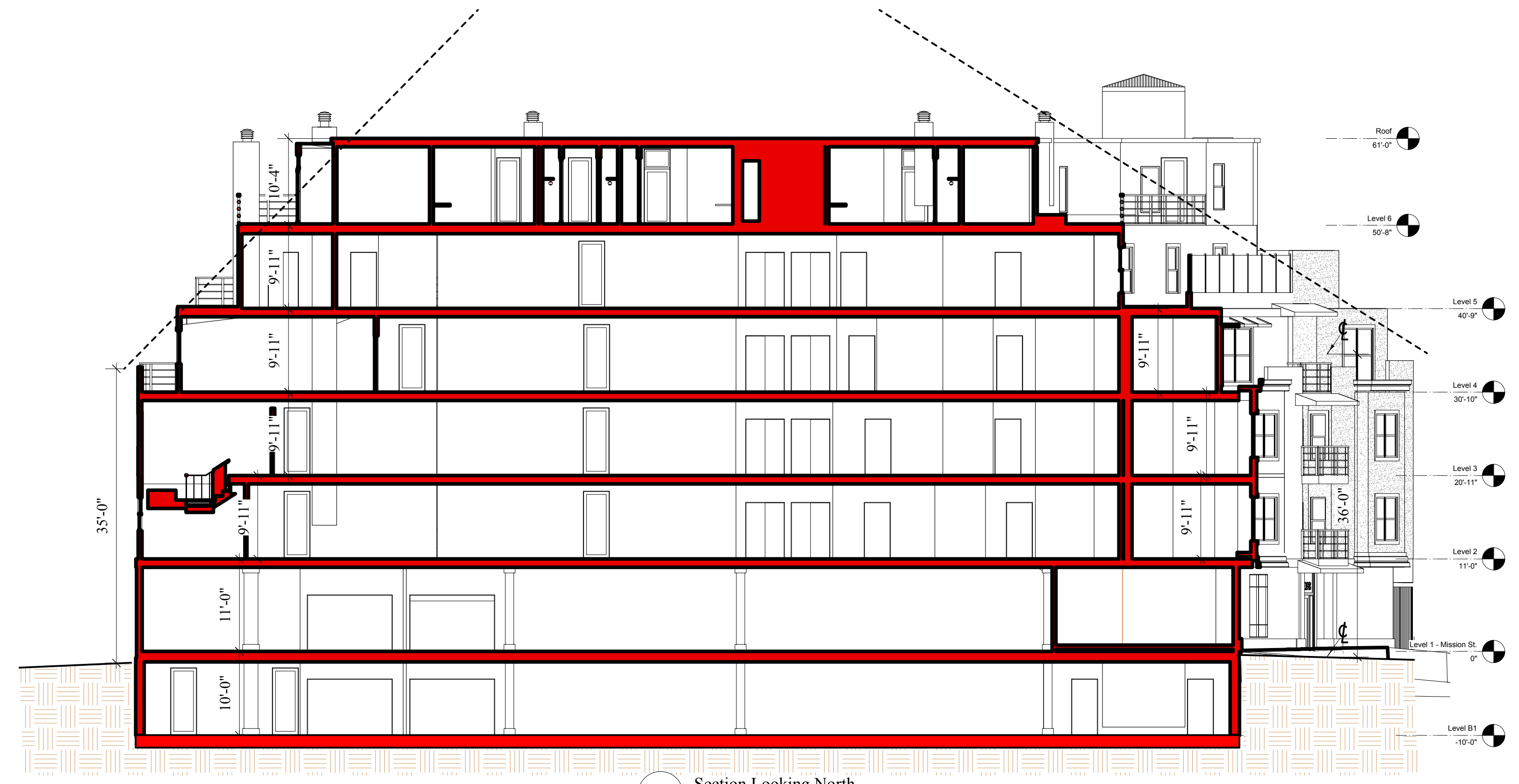
2 Section Looking North Scale: 3/32" = 1'-0"
