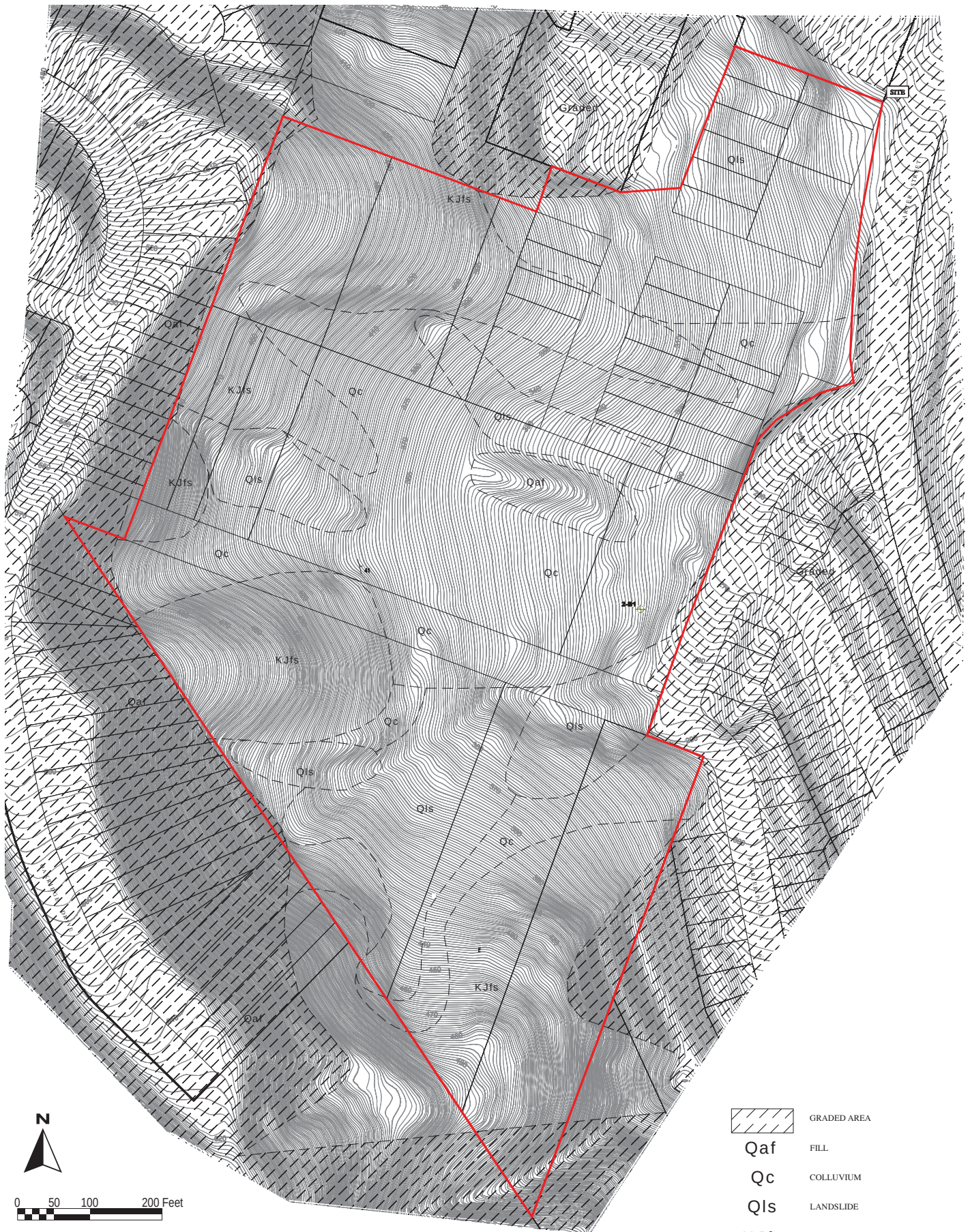
EXISTING SOIL CHARACTERISTICS
