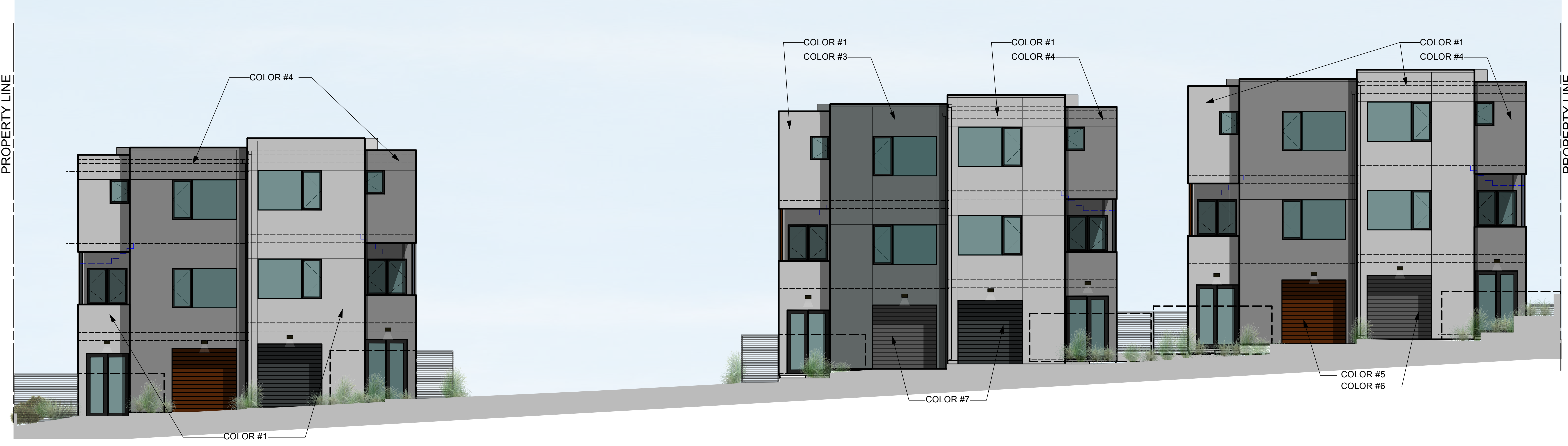
1 PROPOSED EAST ELEVATION (SITE INTERIOR DRIVEWAY) Scale: 1/8" = 1'-0"
