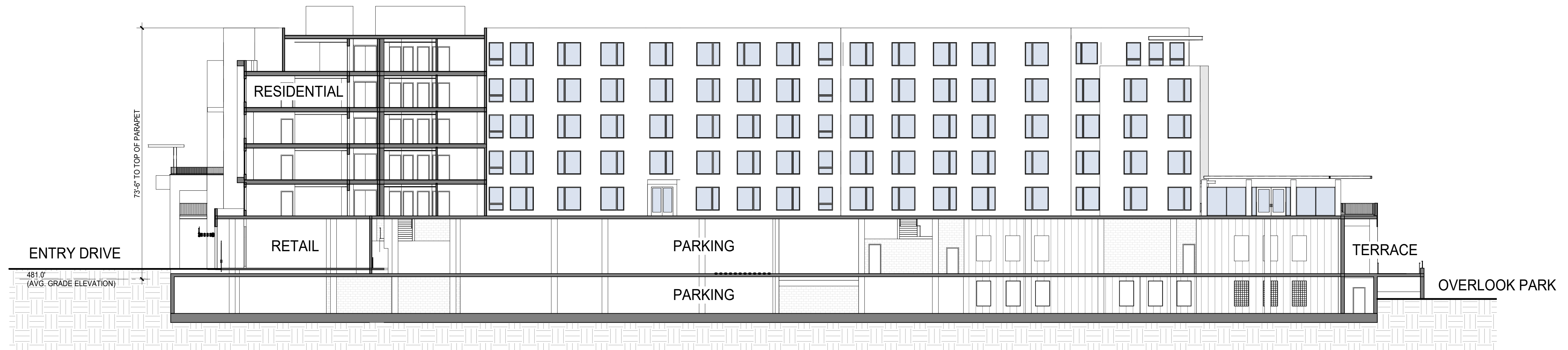
A A4.0 EAST - WEST SECTION (FACING NORTH) 1/16" = 1'-0"
